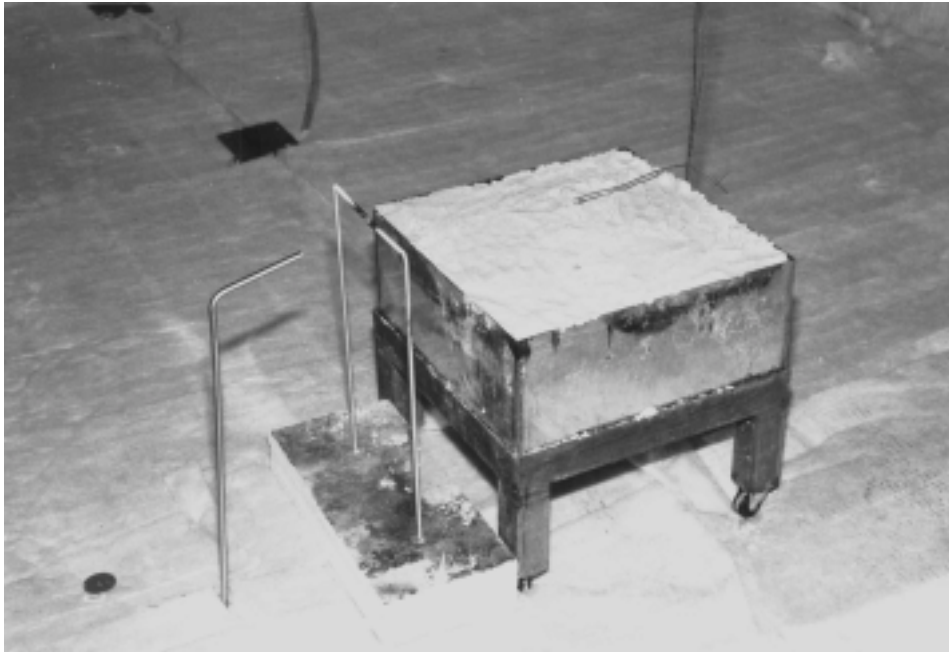
Photo 4-3 The LPG gas burner used in the experiments
