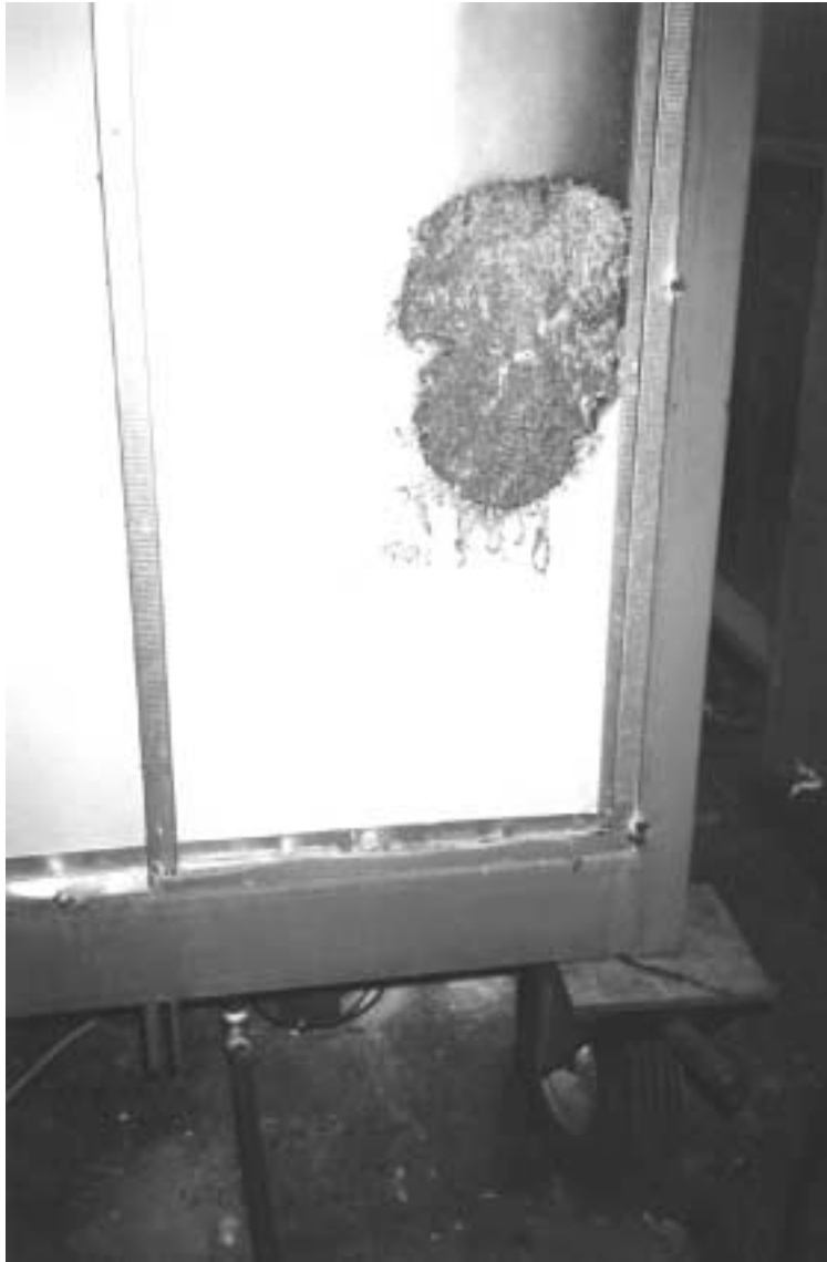
Photo 5-2 Damages to Gib board after 40.5 minutes for run 7
