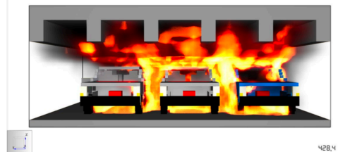
Fig. 24 (Left) Front view – Biggest possible flame of the H2 blowdown captured escaping the bottom of the first car right after the TPRD activation at 7 min. 5 s.
