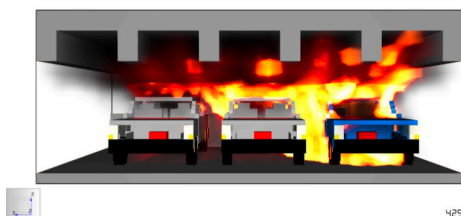
Fig. 23 (Right) Front view – Fire spreads through all the interior of the first car at 3 min. 28 s.
